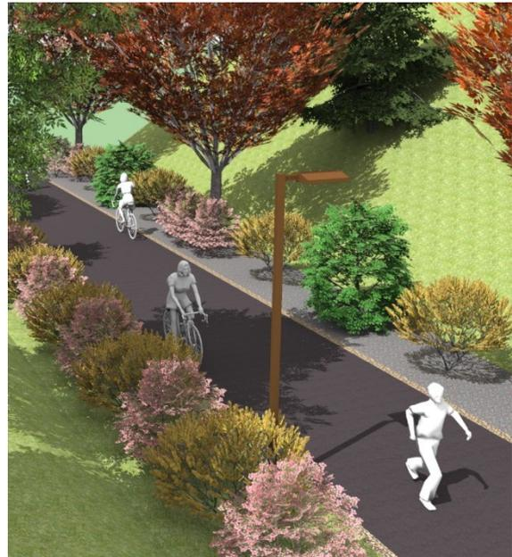
Pole spacing and heights should be appropriate for the particular shared-use path location, and their relative proximity to adjacent uses. A lighting analysis should be completed to prioritize the appropriate corridors, path/road intersections, and amenity areas to determine the areas necessitating lighting, as well as the required illumination levels necessary to create a safe and enjoyable user experience.
